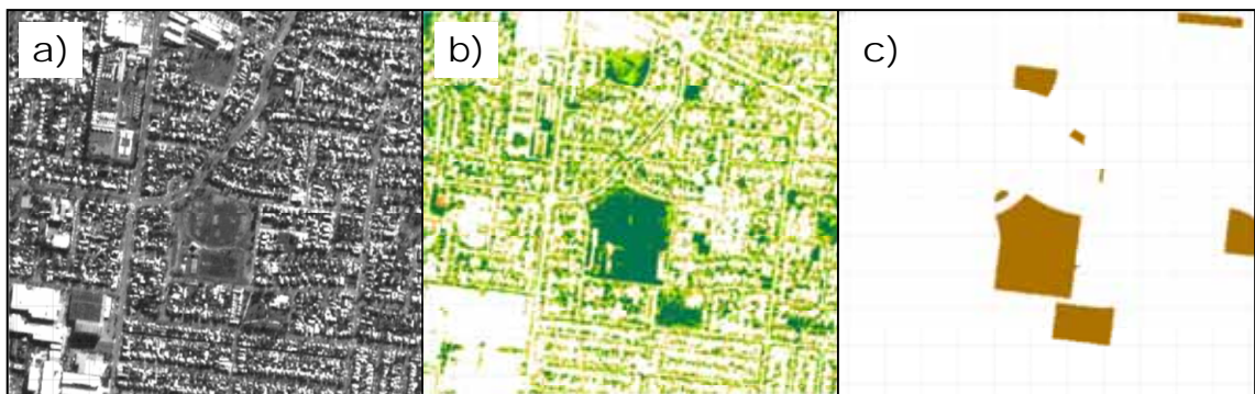
Figure 2: (a) Unclassified remote sensing imagery clearly showing urban infrastructure. Brighter tones associated with high levels of reflectance (such as roofs) and darker areas of vegetation and asphalt surfaces. (b) Remote sensing image classified using the Normalized Difference Vegetation Index (NDVI). Light green areas are irrigated grasses, dark green areas un-irrigated grasses and shrubs, while the tan colour represents tree cover. (c) Designated public open space derived from the cadastre for the same area.
