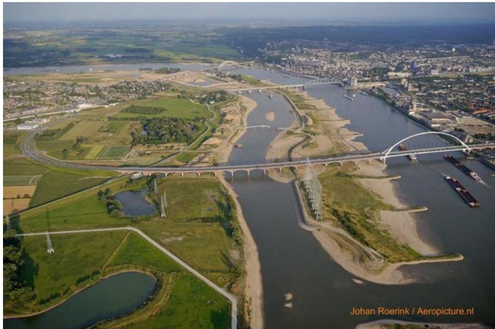
Floodplain redevelopment to accommodate flood waters in Nijmegen, designed by H+N+S Landscape Architects as part of the Room for the River project. Image courtesy of <https://pbs.twimg.com/media/CNMOBiaWIAEJ7Ak.jpg>
